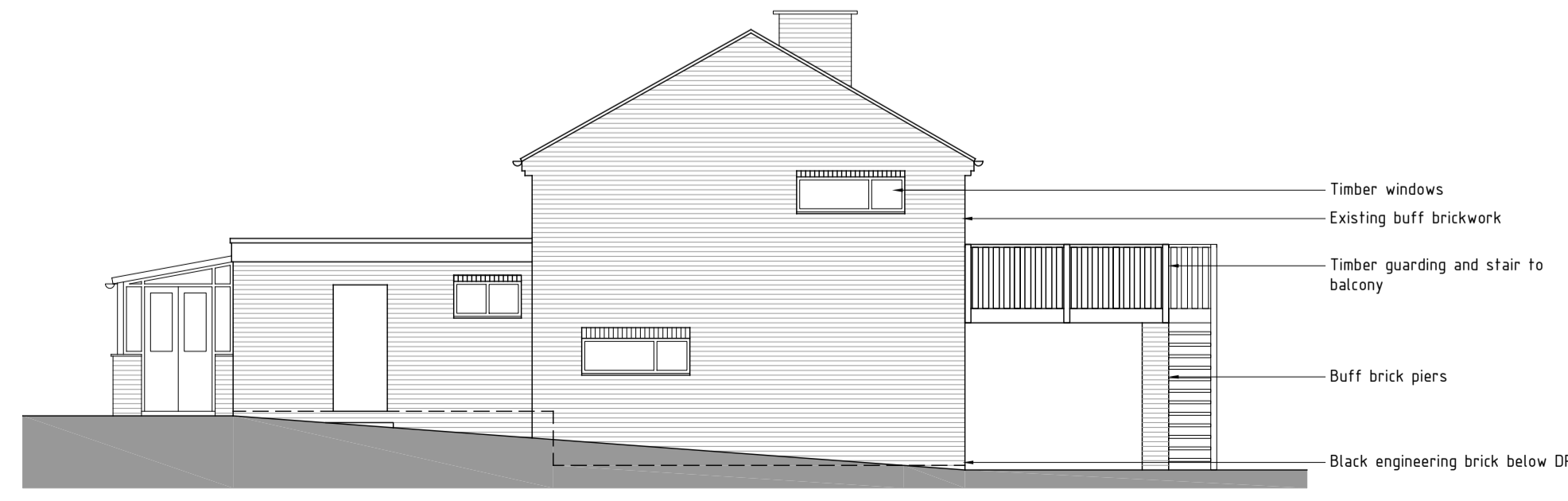
East Elevation as Existing Scale 1:100
